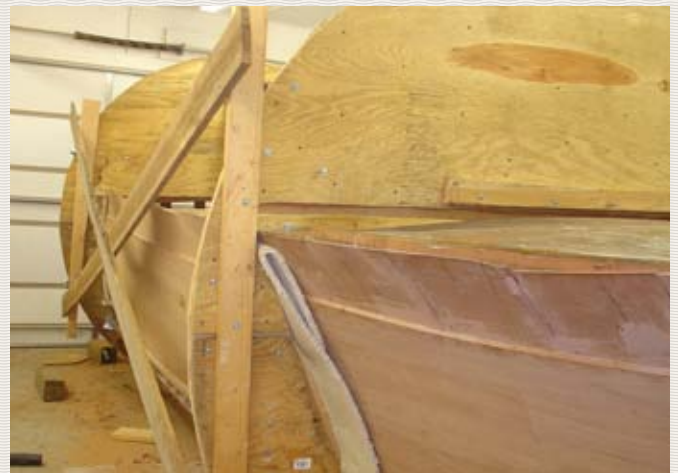
Extra braces added on one side to keep the turning cage better aligned.
